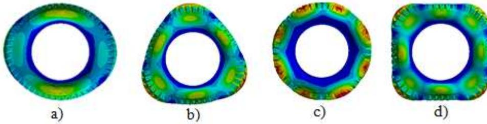
**Figure 3.** Vibration frequencies (f) and deformation (Df) modes of the Tire of light truck
