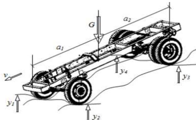
**Figure 2.** Load acting on the wheel of light truck
