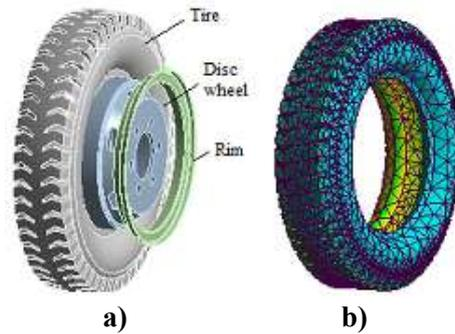
**Figure 1.** Wheel and tire of Light truck
